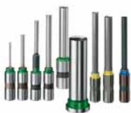
Nagel paper drill bits: 2–35 mm diameter, 50–60 mm working length, and special designs.
